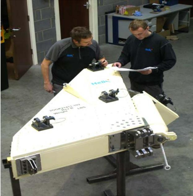
Stovl F35 Joint strike fighter Dummy Tail Assembly fully machined & assembled by Helix Precision.
