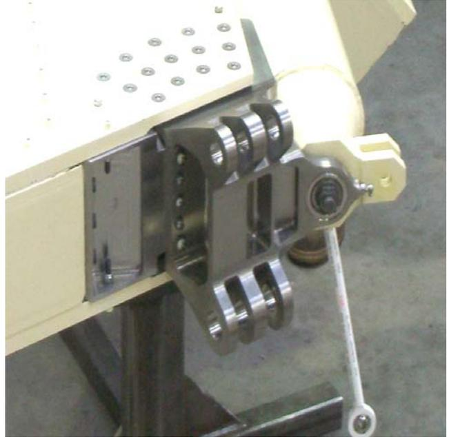
F35 Moment fitting machined from solid Titanium
